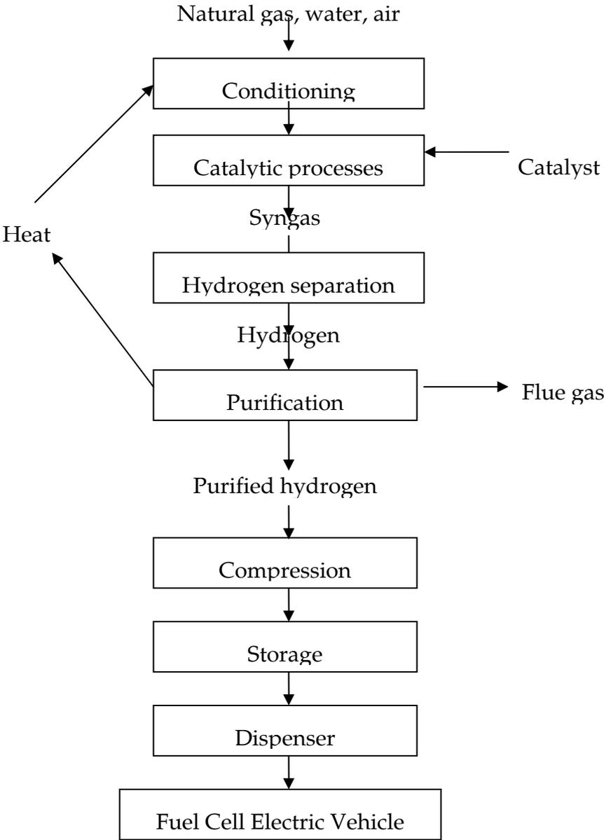
Figure 3. The hydrogen fuel chain at the Mantova project site.
