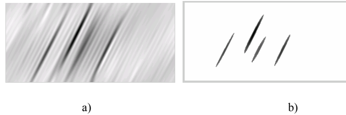
Fig. 3. a) Inverse FT alongside the slope, b) Extraction of the black lines
