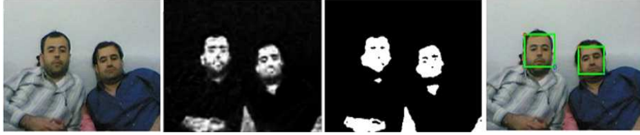
Fig. 2. Face detection process, From left to right: Input color image, its probability and segmented counterpart and detected faces
