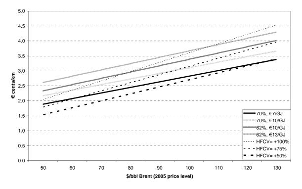
Figure 5. Fuel Cost per Kilometre for alternative Hydrogen Supplies to HFCVs (System efficiency, non-energy costs) and for competing solutions to HFCVs (+efficiency advantage of HFCVs over competing solution).  $\epsilon$ /km.
