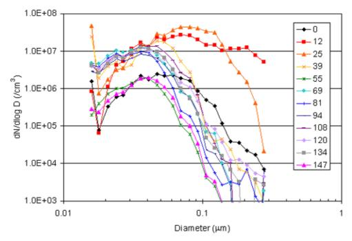
= EA 2002, fig. 60. Aerosol size distributions for AS4013-compliant heater C2, green redgum (water = 33.8%), high flow (sample #39). Values in the legend are minutes after loading fuel.
