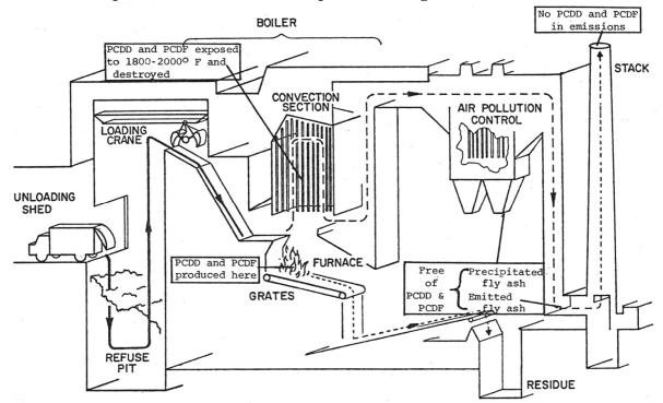
*<u>Fig. 1.</u> Traditional theory of dioxin formation in a MSWI* Source: CBNS 1984, II. Note that dioxins are destroyed by high oven temperatures
